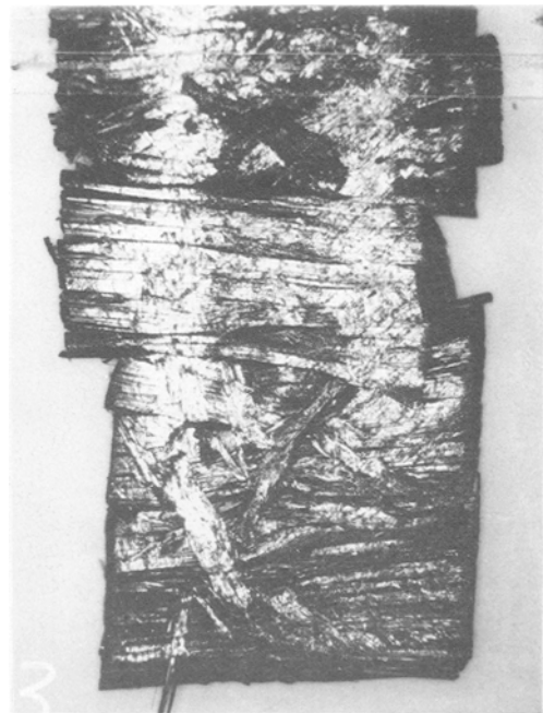
Figure 13 Photograph of a deformed crystal showing a large crack-like shear displacements parallel to the b -axis.
